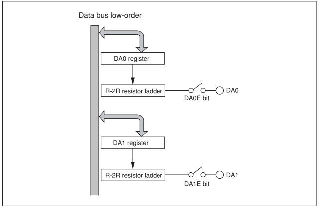
Figure 16.1 D/A Converter Block Diagram
